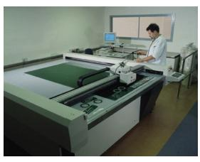
Parts are precision cut by our zero width X-Y CNC. Full CAD/CAM ability means we have no tooling charges (we can work directly from drawings or electronic files) and the delivery lead time is very short. ito15 can also be supplied in sheets or rolls, maximum standard web width = 760mm.
