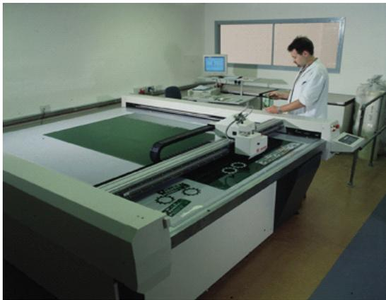
Parts are precision cut by our zero width X-Y CNC. Full CAD/CAM ability means we have no tooling charges (we can work directly from drawings or electronic files) and the delivery lead time is very short. ito15 can also be supplied in sheets or rolls, maximum standard web width = 760mm.
